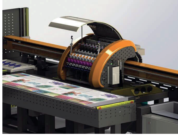
Görüntü 11: Diptech FR-1 modeli dijital dekal baskı makinesi. https://www.dip-tech.com/dinnerware-and-decals
